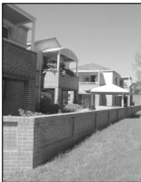
Reduce surface mass of new buildings by providing regular modulation and by using a variety of finished surface details.
