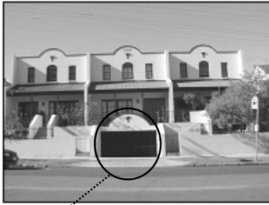
NOT RECOMMENDED: Vehicle entrances to parking areas should not dominate the street elevation.
